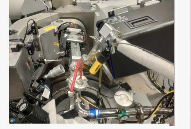
*Combination of 3D computer tomography with tightly focused XRD* (single-crystal or powder) to study micro-inclusions inside bulky matrix
