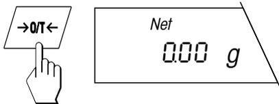
Press the « $\rightarrow 0/T \leftarrow$ » key briefly. The balance is now tared with the additional weight of the new weighing container. If your balance is connected to a printer, the tare weight of the new container is printed out. You can now weigh in additional components.
