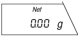
After weighing in of the first component, the display is reset to zero and the balance is now ready for weighing in of the second component.
