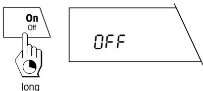
To **switch the balance off**, press the «**On/Off**» key and keep it pressed until the message "OFF" appears in the display.
