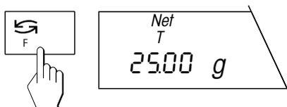
Press the «F» key briefly and the desired weight is confirmed as an additional component.
