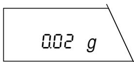
The balance automatically returns to the weighing mode.
