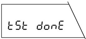
The balance confirms that the test has been performed and then automatically returns to the weighing mode.
