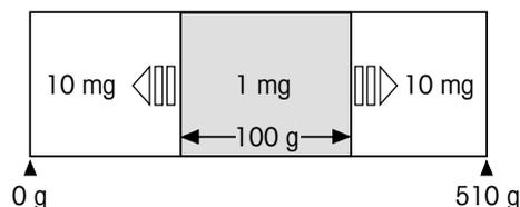
The illustration opposite shows the principle of the movable fine range in which one extra decimal place is shown (in this example, the movable fine range encompasses 100 grams).
