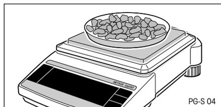
After you have tared the balance, place the weighing sample on the pan.
