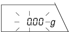
On completion of the adjustment operation, you are prompted to remove the weight. Lift the weight off the weighing pan.
