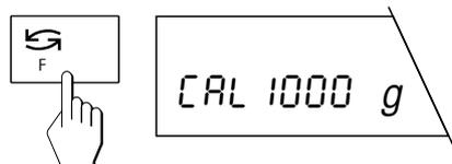
If you do not wish to adjust with the suggested weight, you can select a different weight by pressing the «**F**» key briefly. The available weights depend on the balance model.
