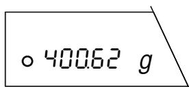
Wait until the circular symbol of the stability detector fades. Fading of the symbol indicates that the weighing result is stable.
