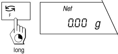
Press and hold the «F» key until the balance switches back to the weight display. You can now weigh in additional components.
