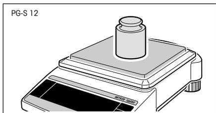
Place the requested weight in the middle of the weighing pan.
