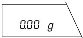
On completion of taring, the zero display appears and your balance is ready for weighing.
