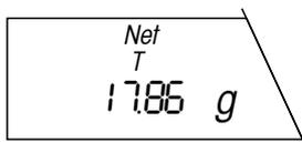
As soon as you have weighed in all components, press the «
