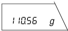
If the fine range in the display is exceeded, the balance display automatically switches to the lower readability.
