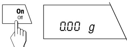
To **switch the balance on**, press the «**On/Off**» key **briefly**. As soon as the normal weight display appears, your balance is ready to weigh.
