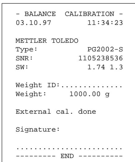
If your balance is connected to a printer, the adjustment is recorded automatically in conformance with GLP. The record shown opposite is a specimen printed with the METTLER TOLEDO LC-P45 Printer. Depending on the attached printer, the printout may differ somewhat from the example shown.
