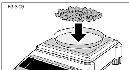
Now add the component to the container until the desired net total weight is reached.
