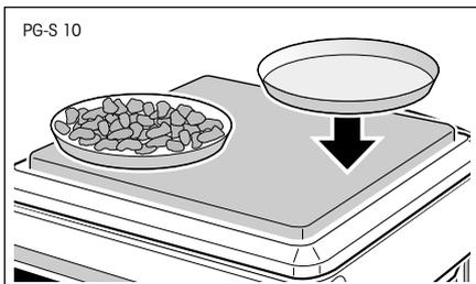
Place the additional weighing container on the weighing pan next to weighing containers already tared.
