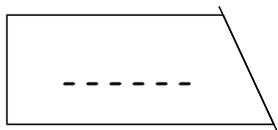
Taring runs automatically. If you tare the balance when it is unstable, the taring procedure will be shown in the display by horizontal segments.
