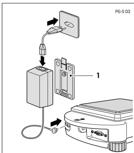
If you wish to work with the holder (1) supplied with the AC adapter: Attach the holder with two screws to a suitable, sufficiently stable area (e.g. on the wall or the underside of a bench top). Press the AC adapter into the holder.
