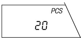
After your balance has determined the reference weight, it shows the correct piece number and is now ready for piece counting.
