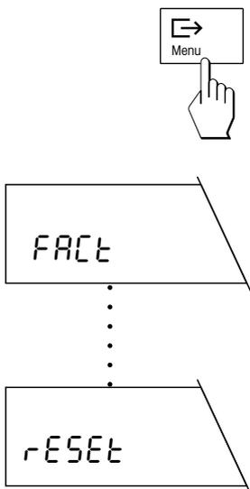
The next menu option appears in the display. Each time the «**Menu**» key is pressed, the balance switches to the following menu option.
