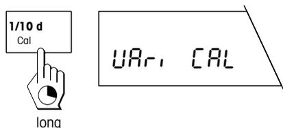
Start the adjustment operation by pressing and holding the «**Cal**» key. The balance shows briefly that adjustment is being performed with external weights.
