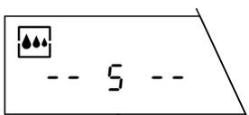
The remaining weighing time (in seconds) is displayed continuously.
