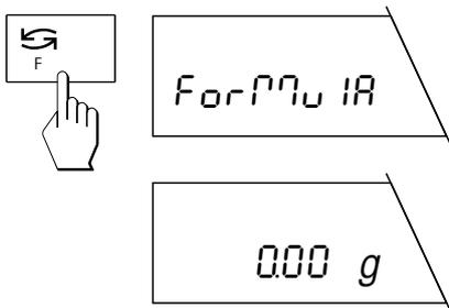
Press the «**F**» key briefly and the display confirms that the formula weighing function is active.
