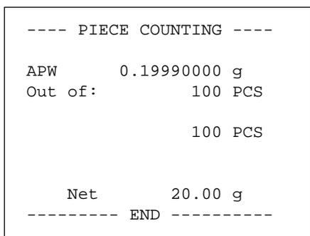
If a printer is connected to your balance, the reference weight, the reference piece number, the total piece count as well as the net weight of the total piece count are printed out.
