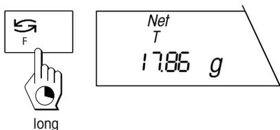
Press and hold the «F» key until the weight of all components weighed in so far is displayed.
