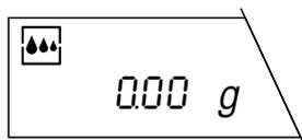
Press the «↻» key briefly. The symbol of the weighing process adapter in the display confirms that dynamic weighing has been activated.
