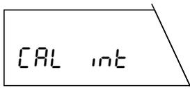
Start the adjustment operation by pressing and holding the «Cal» key. The balance briefly shows that adjustment (calibration) is being performed with the internal weight.
