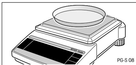
If you are working with a weighing container, place it on the weighing pan in the normal weighing mode.
