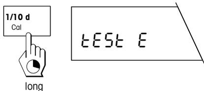
Initiate the test procedure by pressing and holding the «Cal» key. The balance briefly confirms that the test is being performed with an external weight.
