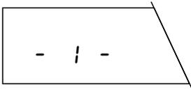
Then press the «
