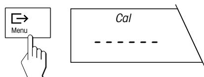
Confirm the selected weight with the «**Menu**» key. This initiates the adjustment process. The balance determines the zero point.
