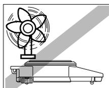
No excessive drafts (powerful air conditioning systems or fume hoods can also cause drafts).
