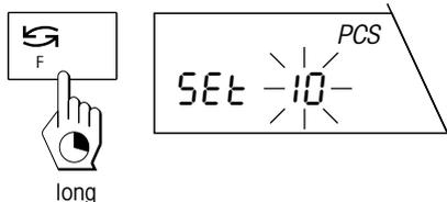
Your balance now needs the weight of a **reference piece number**. Press and hold the «F» key until you are prompted to load the reference pieces.
