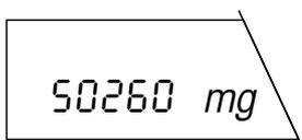
The balance shows the result in **weighing unit 2**. By pressing the «
