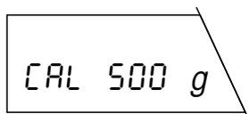
The balance now prompts you to select the desired weight. If you do not press a key for 3 seconds, the balance automatically initiates the adjustment process.
