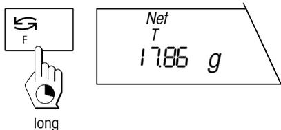
Press and hold the «F» key until the net total weight of all components weighed in so far is displayed.
