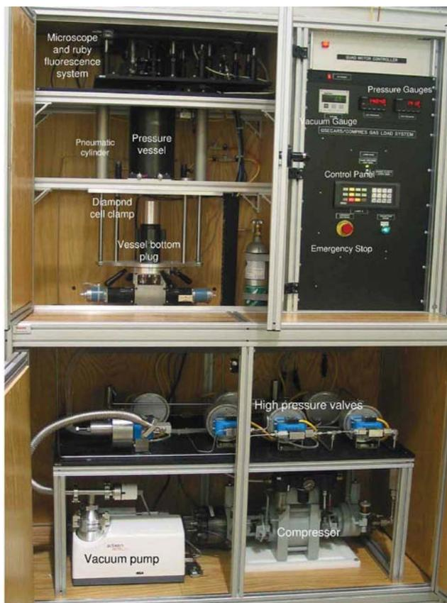
Figure 3. Annotated photograph of the system. The four doors are open to show the interior of the cabinet. The control computer and the large gas cylinder are not shown.
